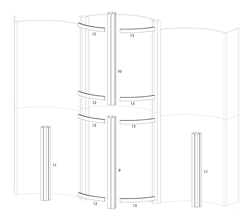
Place and attach Custom Headers to Backwall as shown at right.
