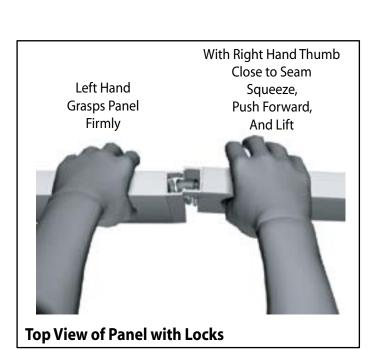
The first level of components contains panel locks that are located at the top of the panel for extra stability and a seamless connection. When disassembling panels, twist top connection slightly and lift right panel upward.
