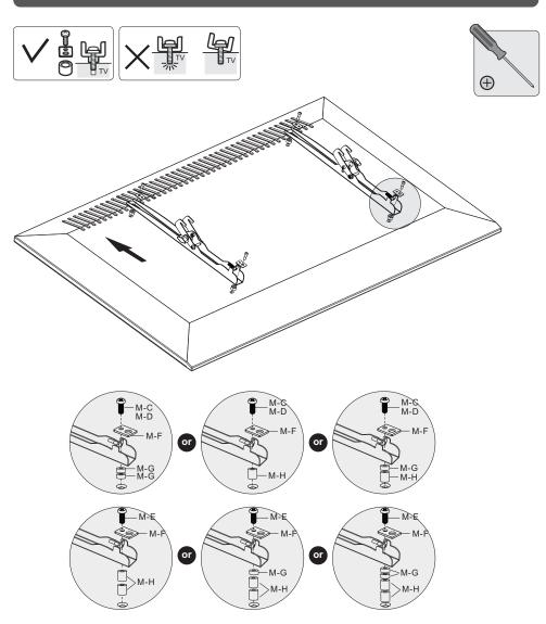
Note: Choose the appropriate screws, washers and spacers (if necessary) according to the type of screen. Position the adapter brackets as close as possible to the center of the TV.
