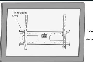
Use the tilt adjusting knob to adjust your TV to the desired angle.
