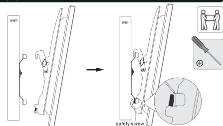
Hook the TV over the top of the wall plate. Tighten the safety screws on the display brackets with a proper screw driver.
