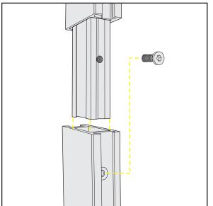
Inline Connection between Extrusions
