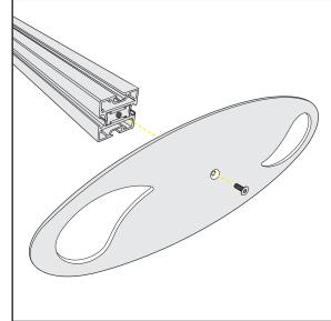
Baseplate Connection for Vertical Extrusions
