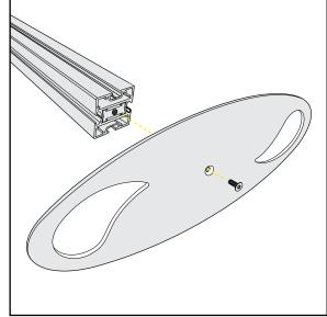
Baseplate Connection for Vertical Extrusions
