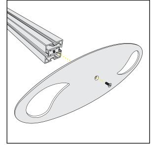
Baseplate Connection for Vertical Extrusions
