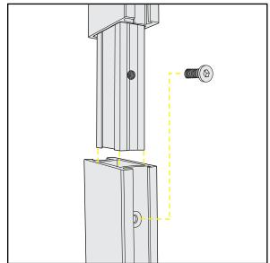
Inline Connection between Extrusions
